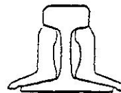
80-lb. A.S.C.E. RAIL 80 lbs per yard Stock lengths 30' and 39' Joint bars 24' length 48' lbs per bar Track bolts 7/8" x 4" with heavy square nuts
