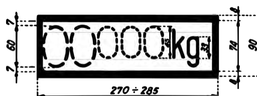
Figure 2: Wagon tare and braked weight of the platform-operated hand brake
