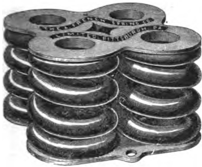
Fig. 5205. BOLSTER-SPRING. Four single-coil springs. Diameter of case, 11 ins. Height, 6 ins. Capacity, 6 to 8 tons.
