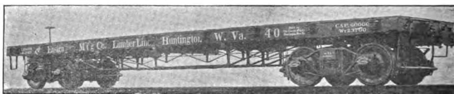
Fig. 19. FLAT CAR. FOR BRIDGE TIMBERS. Length, 41 ft. Capacity, 60,000 lbs. Weight, 23,700 lbs. Equipped with Rigid Diamond Trucks (Details are shown in Figs. 294-297.)
