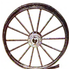
Figs. 5626-5628 THE CYRUS ROBERTS STEEL-TIRED WHEEL. Cast Hub, Steel Spokes and Felloe and Steel Flanged Tires. New tires may be shrunk on to center.
