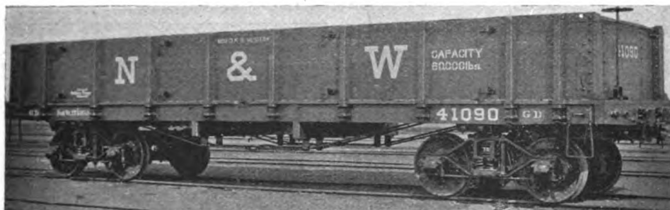
Fig. 23. GONDOLA CAR, WITH DROP-BOTTOM AND DROP-ENDS, FOR COAL, ORE AND LUMBER
