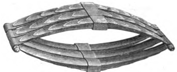
Fig. 5233. CONCAVE ELLIPTIC-SPRING. (36 in. \times 12 \frac{1}{4} in. high, 6 leaves ; main, 3 \times \frac{1}{4} in.; others, 3 \times 3-16 in. Weight, 183 lbs. Capacity, 9,500 lbs., half exhausted.)
