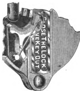
Fig. 2765. Showing manner in which escutcheon drops into place.
