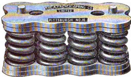
Fig. 5221. BOLSTER-SPRING OF 8 SINGLE COILS. Width of Case, 7½ ins. Capacity, 5 to 6 tons.
