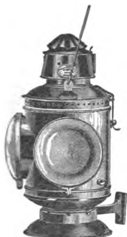
Fig. 3318. ENGINE-LAMP WITH TWO LENSES.
