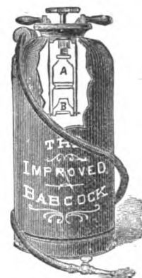
Fig. 3704. BABCOCK FIRE- EXTINGUISHER. A. Acid-bottle. B. Acid-bottle Carrier.
