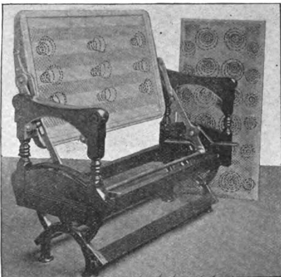
Fig. 3953. Sectional View. Showing Construction and Mechanism. HIGH-BACK TILTING CAR-SEAT.
