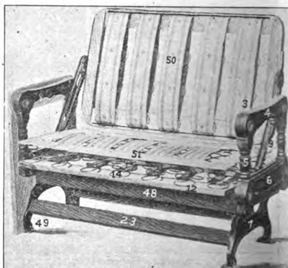
Fig. 3923. No. 73. CAR SEAT IN PROCESS OF CONSTRUCTION With Steel Top Spring-edge Cushion and Back.
