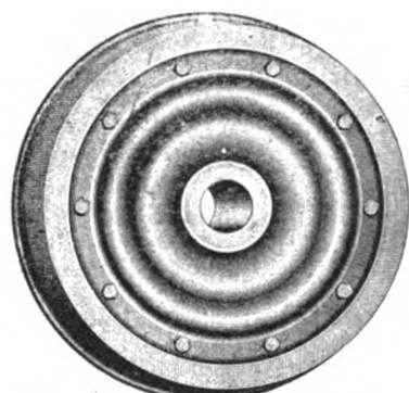
Figs. 5259-5260. No. 11. Wheel with Cast-iron Double-plate Center. Tire secured by One Retaining-ring.
