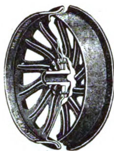
Figs. 5620-5621. THE BUDA CORRUGATED STEEL WHEEL. THE BUDA STEEL WHEEL.* *The Tread and Web of Wheel are formed by Drawing and Spinning a Single Plate of Steel.
