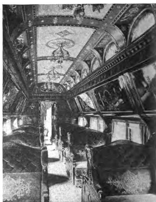
Fig. 126. INTERIOR OF SLEEPING CAR AMERICA. Exhibited at World's Columbian Exposition, 1893, by Pullman's Palace Car Company. Vaulted Ceiling, Oval Deck-Windows, Disappearing Curtain Rods and Electric Lights. (Plan is shown in Fig. 186.)
