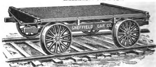
Fig. 5604. PUSH-CAR. Platform, 7 ft. \times 5½ ft. Weight, 470 lbs
