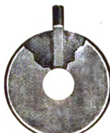
Figs. 5626-5628 THE CYRUS ROBERTS STEEL-TIRED WHEEL. Cast Hub, Steel Spokes and Felloe and Steel Flanged Tires. New tires may be shrunk on to center.
