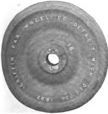
Figs. 5337-5338. CHILLED CAST WHEEL, With curved ribs or brackets.
