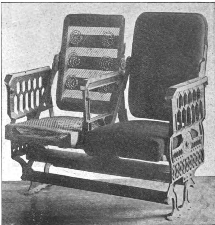
Fig. 3955. Sectional View. DOUBLE OR TWIN CAR-SEAT. WITH DIVISION-ARM.
