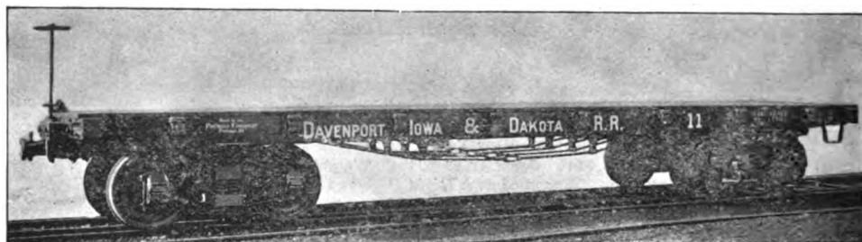
Fig. 18. FLAT CAR. DAVENPORT, IOWA & DAKOTA RAILROAD. Length, 34 ft. Capacity, 60,000 lbs. Weight, 17,700 lbs. Equipped with Rigid Diamond Trucks.
