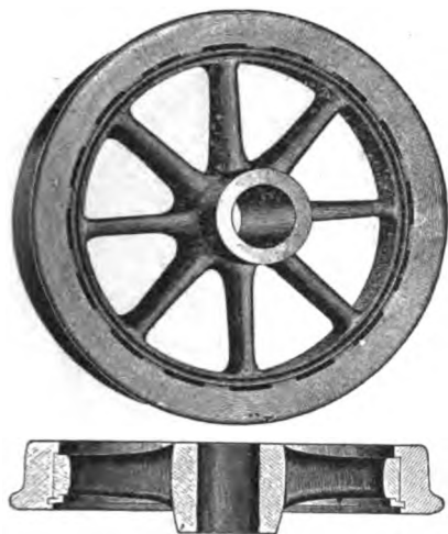
Figs. 5292-5293. SOLID SINGLE-OVAL-SPOKE WHEEL. Brunswick Tire-fastening.
