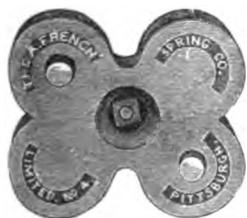
Fig. 5214. NARROW-GAGE BOLSTER-SPRING. Width of case, 7 ins. Four two-coil springs. Capacity, 2 tons.
