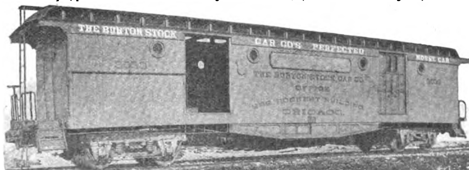
Fig. 45. STOCK CAR FOR HORSES AND PRIZE CATTLE. THE BURTON STOCK CAR COMPANY. Length, 44 ft. Capacity, 16 horses, or 22,400 lbs. (Interiors shown in Figs. 46 and 47.)
