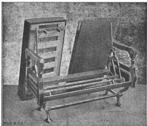
STANDARD COACH SEAT. Seat is taken apart, to show mechanism.
