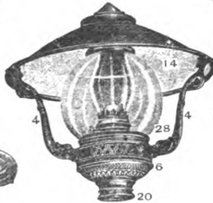
Fig. 3311. VESTIBULE OR PLATFORM LAMP. Drop, 16 ins. Enameled reflector.
