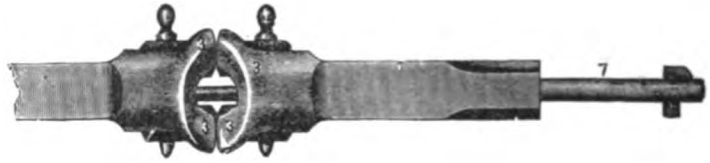
Fig. 2074. Link and Pin Coupler. Malleable cast iron.
