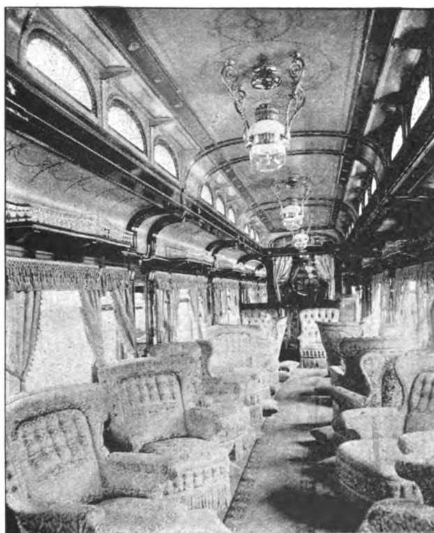
Fig. 116. INTERIOR OF PARLOR CAR MAUD. Cornice Bracketed to Support Basket Racks, Pintsch Light and Bay Windows. (Exterior is shown in Fig. 115.)
