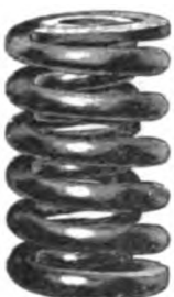
Fig. 5235. 5 \frac{1}{4} \times 8 ins. DRAFT-SPRINGS, 2-COIL.
