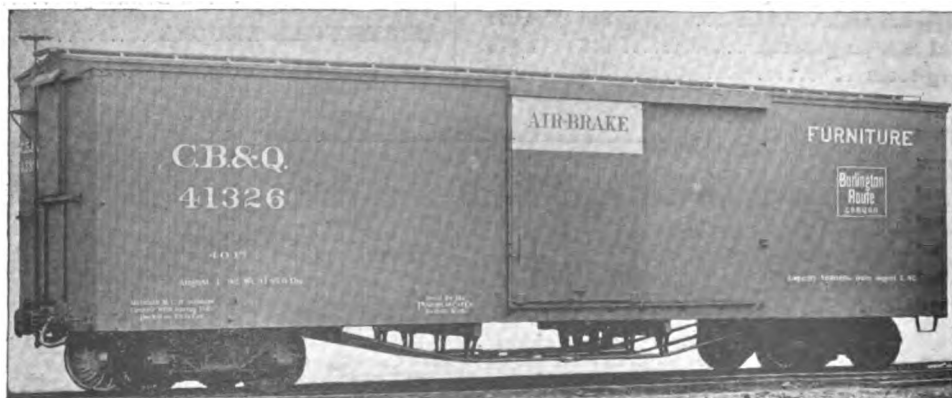
Fig. 4. FURNITURE CAR. CHICAGO, BURLINGTON & QUINCY RAILROAD. Length, 40 ft. Capacity, 50,000 lbs. Weight, 31,850 lbs. Coupler is placed between Center Sills to get greater height of Car-body. (Details are shown in Figs. 247-250.)
