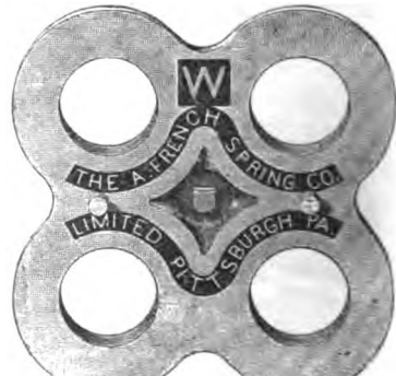
Figs. 5203-5204. BOLSTER-SPRING. Four single-coil springs. Diameter of Case, 11 ins. Height, 7 ins. Capacity, 6 to 8 tons. (352)
