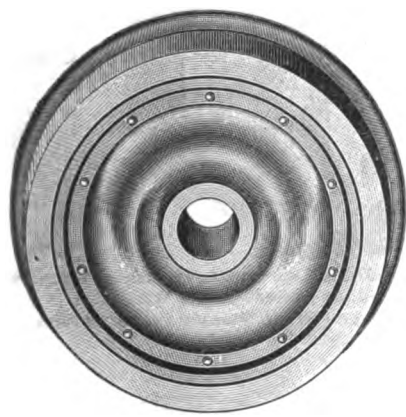
Figs. 5302-5303. NO. 1 WHEEL. Wrought-iron Coil-disc Centre. Tire Secured by Wrought-iron Retaining-rings.
