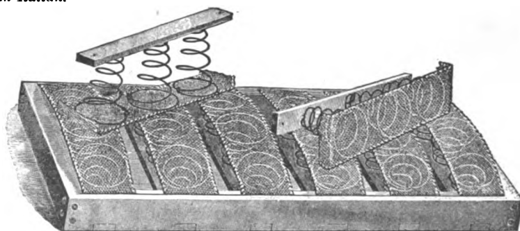
Fig. 3956. SEAT CUSHION AND DETACHED SECTIONS. Showing Construction. ROBERTS' PATENT WOVEN-WIRE CAR SEATS.
