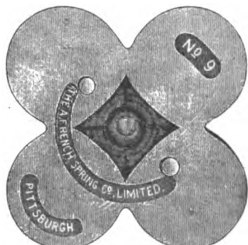
Figs. 5201-5202. BOLSTER-SPRING. Four springs in groups of 3 coils or less, as required. Width of Case, 11 ins. Capacity, 5 to 8 tons.
