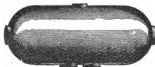
Fig. 2903. CIRCULATING DRUM, OR WATER RESERVOIR AND EXPANSION CHAMBER.
