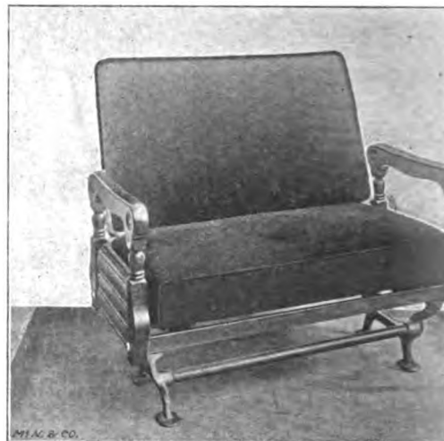
STANDARD COACH SEAT. Length over all, 40 ins. Height of back, 24 ins.
