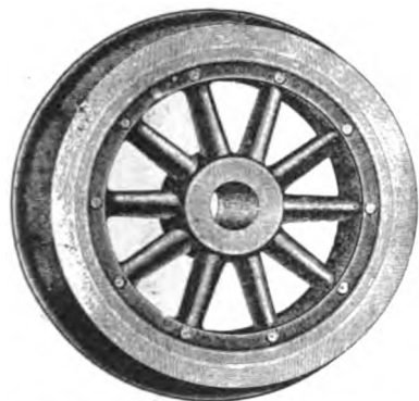
Figs. 5255-5258. No. 1. Wheel with Paper Center. Tire secured by Plates and Bolts.
