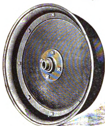
Figs. 5632-5634. KALAMAZOO ALL-STEEL HAND-CAR WHEEL. Malleable-iron Flanged Hub, Double Steel-plate Center, Wood Felloe, Re-enforced with Steel Rings.
